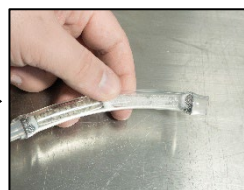
3. Break the glass capsules in the smoke test ampulla.
