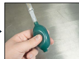
4. Pump with the hand pump a few times to push smoke into the sensor.
