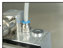
2. Connect the smoke test adapter to the inlet.
