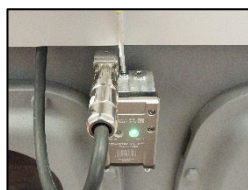
1. Unscrew the oil mist test inlet on the top of the sensor.
