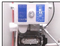
15. Connect the scavenging air hose from the measuring head to the injector on the baseplate.
