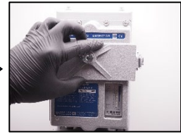
4. Close inspection cover.
