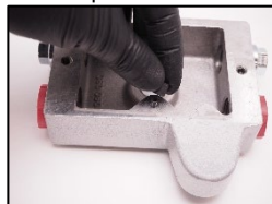
5. Check the small seal.
