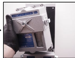
3. Dismount the measuring head.
