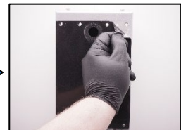
12. Change the measuring head seal.
