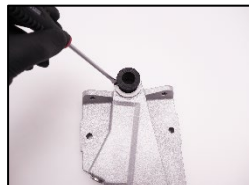
10. Change the flexible bellows.
