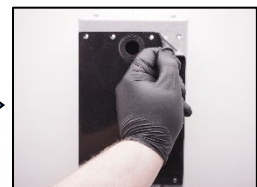
12. Change the measuring head seal.
