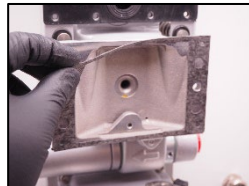
6. Change the valve box seal.
