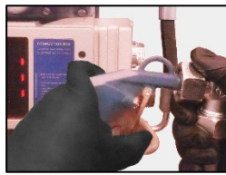
2. Use compressed air to blow back collected oil into the engine.
