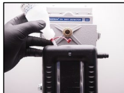
2. Fill in slacked water in the u-tube manometer to the middle line.
