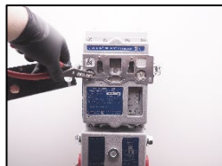
2. Using circlip pliers, change the scavenging air filter.
