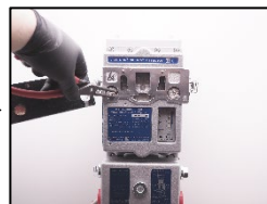
15. Change the scavenging air filter.
