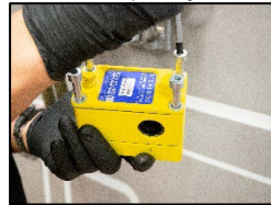
11. Tighten the screws until the siphon block holds together.
