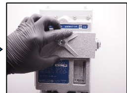
20. Close inspection cover.
