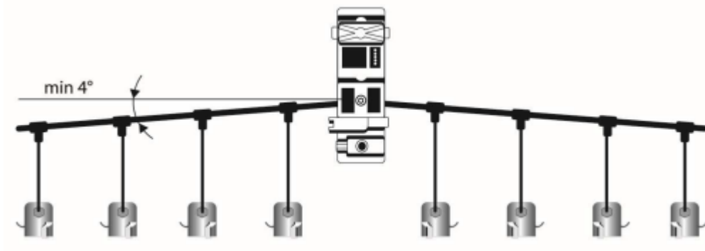
Typical pipe system installation.
