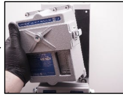
3. Dismount the measuring head.
