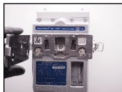
14. Open the inspection cover.
