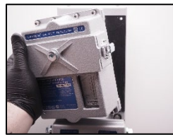
3. Dismount the measuring head.
